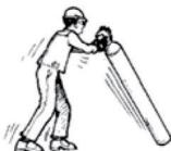
Lift decisively with a smooth non-jerking motion. It is done initially by straightening the legs then following through with the arms at the same time walking forward until the cylinder is upright.
