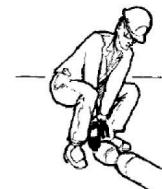
Ensure that the valve guard is secure then take a firm grip using both hands. Only lift using the guard if it has been designed for this purpose, otherwise grip the cylinder neck.
