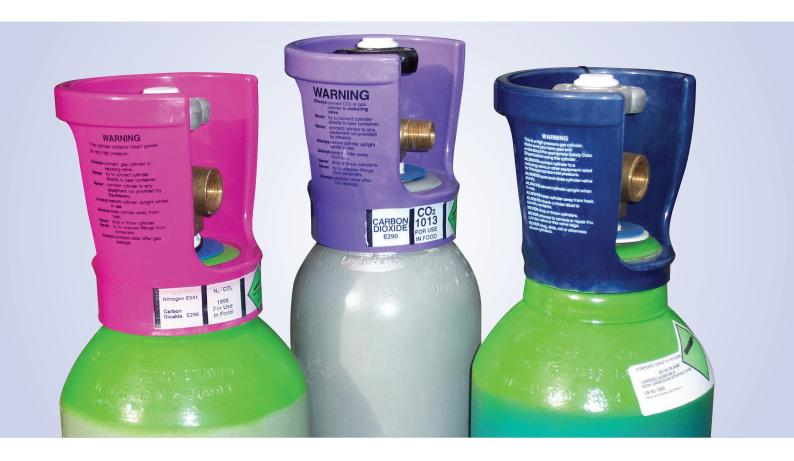
The plastic cylinder valve guard protects valves from accidental damage and is for use on all Industrial Gas cylinders up to 50 kg gross filled weight (Nylon) and 35 kg (ABS plastic).
