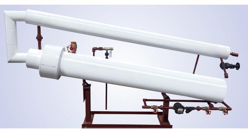
Steam heated vaporisers provide an easy and cost effective method of vaporising large quantities of liquid  $CO_2$  to gas. Designed for direct connection to the outlet of a bulk storage tank, the steam vaporisers are available with nominal vaporisation capacities of 0.5 te/h, 1.0 te/h and 2.0 te/h.
