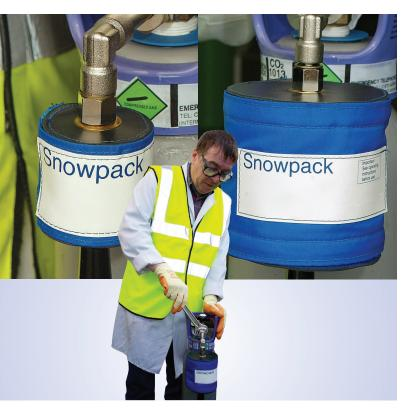
The Snowpack makes individual pellets of dry ice from a carbon dioxide syphon cylinder, which has an internal dip tube.
